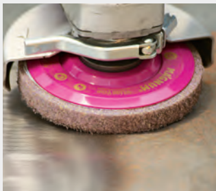
Steel: Fine grinding, deburring, rust removal
