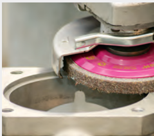
Aluminium: Cleaning, fine grinding
