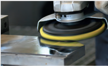
Subsequent mirror finish polish with the BRIGHTEX® polishing system (Berry + Sun).
