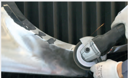
Removes paint while achieving a surface finish.
