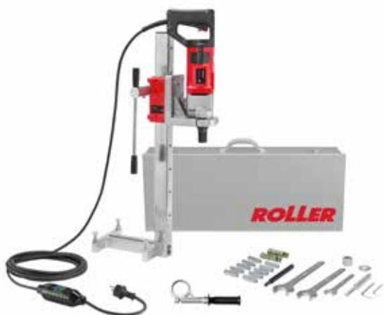
**Universal, powerful, robust, handy diamond core drilling machine for core drilling, for example in concrete, steel-reinforced concrete up to Ø 102 (132) mm, in masonry of all kinds, natural stone, asphalt, screeds of all kinds, up to Ø 162 mm. For dry or wet drilling, hand held or with drill stand.**
