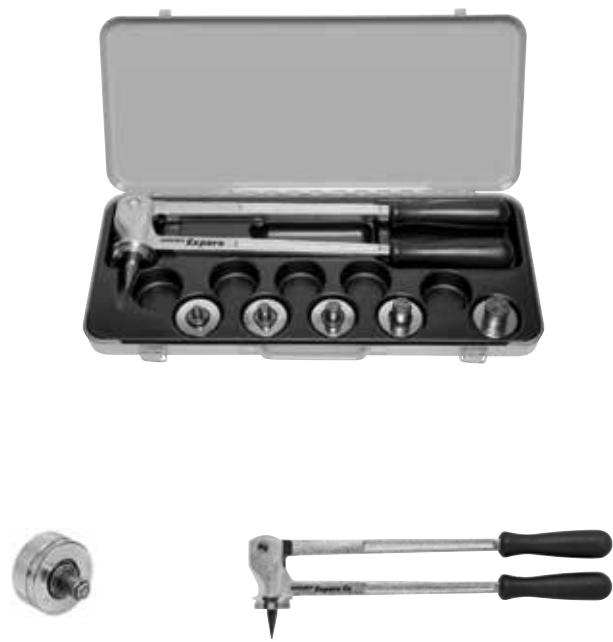
**Robust, stable manual tube expander for soft copper tubes Ø 8–42 mm, Ø ½–1½", wall thickness up to 1.5 mm, soft aluminium and precision steel tubes Ø 8–42 mm, wall thickness up to 1.2 mm, soft, stainless steel tubes Ø 8–42 mm, wall thickness up to 1 mm.**
