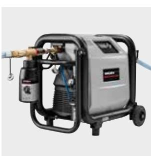
**Powerful, compact, electronic flushing unit with oil-free compressor.** For flushing with water/air mixture, disinfection, cleaning, preservation of pipe systems. Flushing and desilting of pipes up to DN 50, Ø 2" with a water pressure pipe network up to 1 MPa/10 bar/145 psi. Water temperature 5–35°C, water flow up to 5 m³/h. Operation of pneumatic tools with an operating pressure up to 0.8 MPa/8 bar/116 psi, suction power up to 230 Nl/min.
