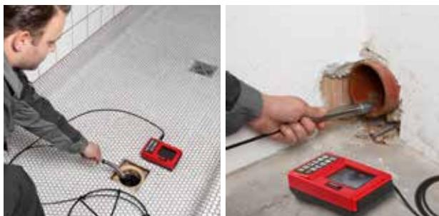
**Very compact, lightweight, electronic camera inspection system for brilliant pictures and videos of pipes and drains Ø 40 – 150 mm, chimneys and other hollow cavities.**
