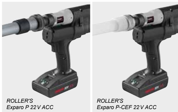
**Ultra-handy, ultra-light, robust 20 kN hybrid pipe expander for cordless and mains operation, with automatic return (ACC). For expanding pipes/rings. Optionally with Cu, P or P-CEF expander. Li-Ion 22 V Technology! Li-Ion 21.6 V, 2.5 Ah battery for approx. 600 expansions per battery charge\*.**
