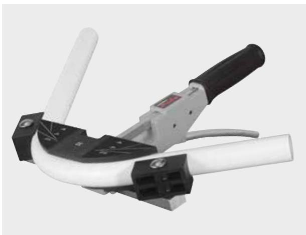
**Practical, ultra handy, ultra light compact one-handed pipe bender for soft copper pipes Ø 10–22 mm, Ø  $\frac{3}{8}$ – $\frac{7}{8}$ ", s ≤ 1.0 mm, soft jacketed copper pipes Ø 10–18 mm, Ø  $\frac{3}{8}$ – $\frac{7}{8}$ ", s ≤ 1.0 mm, soft coated carbon steel pipes of the press fitting systems Ø 12–18 mm, s ≤ 1.2 mm, soft precision steel pipes Ø 10–18 mm, s ≤ 1.0 mm. Multi-layer composite pipes Ø 14–32 mm. (s = wall thickness)**
