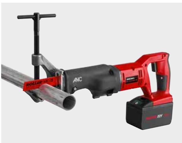
**Powerful, robust, compact hybrid pipe saw for cordless and mains operation. Ideal for steel pipes and other pipes as well as for many materials, e.g. wood, wood with nails, pallets, metal, also stainless steel, cast iron, breeze blocks, plaster boards etc. Li-Ion 22 V Technology! Li-Ion 21.6 V, 9.0 Ah battery for approx. 80 1" steel pipe cuts with guide holder per battery charge\*.**
