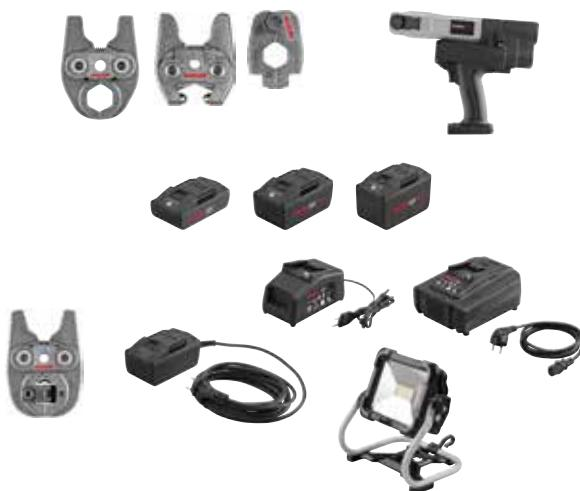
**Ultra-handy, ultra-light, robust hybrid radial press 22 kN for cordless and mains operation, with automatic circuit control. For radial press joints Ø 10–40 mm, Ø ¼–1 ¼". Li-Ion 22 V Technology! Li-Ion 21.6 V, 2.5Ah battery, for approx. 390 pressings per battery charge\*.**
