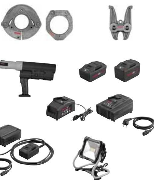
**Powerful, universal, robust hybrid radial press XL 45 kN for cordless and mains operation with automatic circuit control. Antivibration system. For radial press joints XL Ø 64–108 mm, Ø 2½–4". Li-Ion 22 V Technology! Li-Ion 21.6 V, 5.0 Ah battery for approx. 150 pressings per battery charge\*.**
