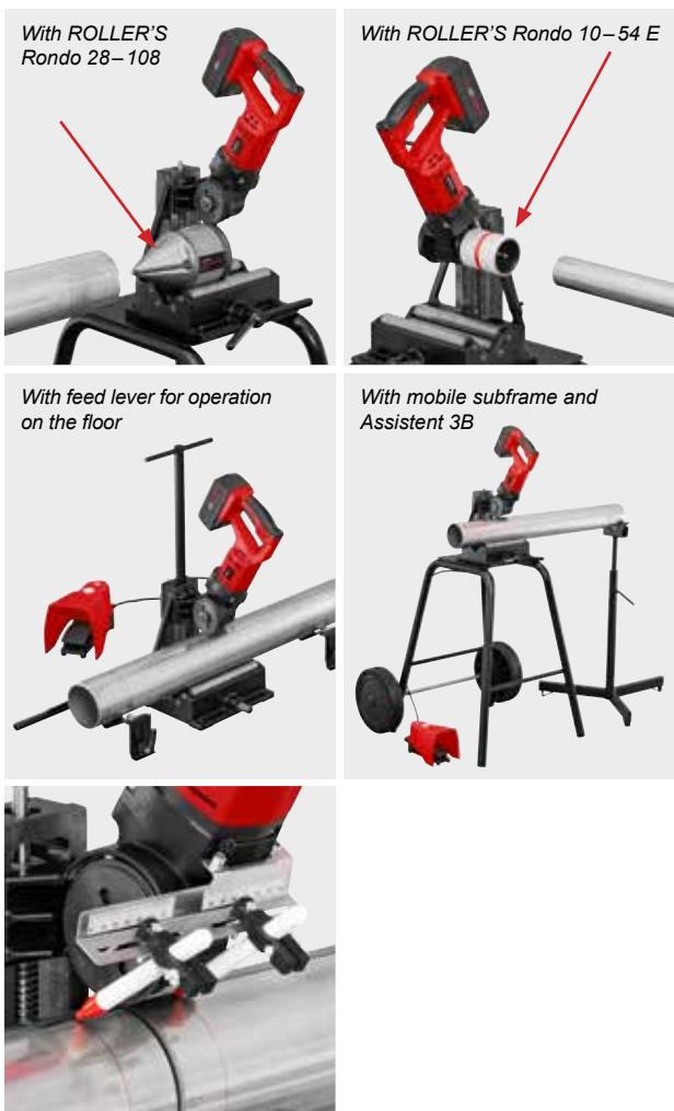
**Compact, light, robust hybrid pipe cutting machine for cordless and mains operation. For mobile cutting and deburring pipes of the press fitting systems made of stainless steel, copper, carbon steel, Ø 8–108 mm, steel pipes EN 10255 (DIN 2440) DN 6–100, Ø ½–4", Ø 10–115 mm, cast iron pipes (SML) EN 877 (DIN 19522) DN 50–100, plastic pipes SDR 11 wall thickness s ≤ 10 mm, Ø 10–110 mm, composite tubes Ø 10–110 mm. Li-Ion 21.6 V, 5.0 Ah battery for approx. 280 cuts Ø 22 mm per battery charge\*.**
