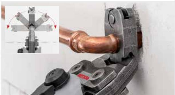
**Example: ROLLER'S Mini V pressing tongs: Impression "V"**
