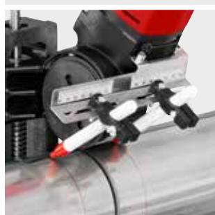
**Compact, lightweight, robust pipe cutting machine for cutting and removing burr from pipes of the pressfitting systems of stainless steel, copper, C-steel, Ø 8–108 mm, steel pipes EN 10255 (DIN 2440) DN 6–100, Ø ½–4", Ø 10–115 mm, cast iron pipes (SML) EN 877 (DIN 19522) DN 50–100, plastic pipes SDR 11 wall thickness s ≤ 10 mm, Ø 10–110 mm, Ø ¼–4", composite tubes Ø 10–110 mm. ROLLER'S Disc 100 RF for welded drain pipe/down pipe made of stainless steel EN 1124 Ø 40–110 mm**
