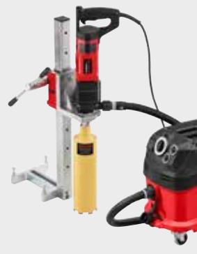
**Powerful, robust, handy diamond core drilling machine with micro-pulse technology.** For core drilling without water, e.g. in concrete, steel-reinforced concrete up to Ø 162 (202) mm, in all kinds of masonry, natural stones, asphalt, all kinds of screed, up to Ø 202 mm. Especially for dry drilling, hand held or with drill stand.
