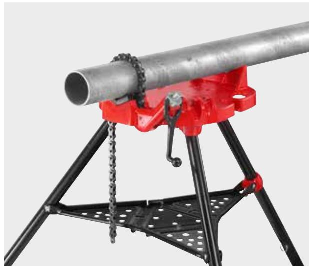
**Robust pipe processing station with integrated chain pipe vice on collapsible tripod stand. For clamping pipes, solid material Ø ½–6", 10–165 mm. Load capacity up to 450 kg.**
