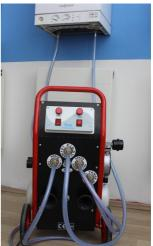
"dump outlet "and lead the hose to a toilet pan or drain pipe gully leading to a foul sewer.
